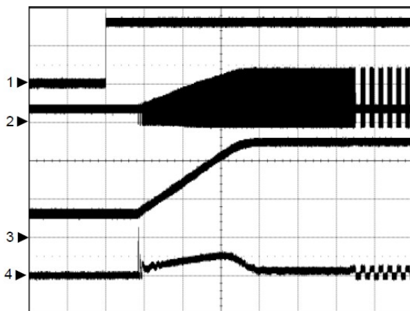
Start-up at PSM Condition
