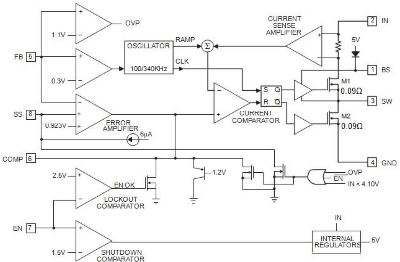
Figure 3 Function Block Diagram of EC3286
