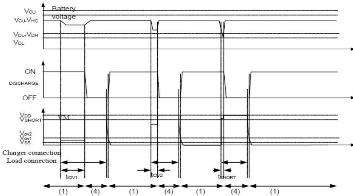
Remark: (1) Normal condition (2) Over-charge Voltage condition (3) Over-discharge Voltage condition (4) Over Current condition
