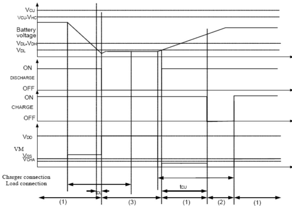
Remark: (1) Normal condition (2) Over-charge Voltage condition (3) Over-discharge Voltage condition (4) Over Current condition
