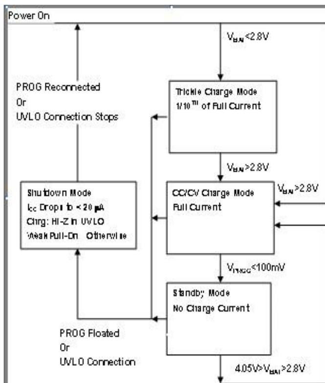
Figure 1. State Diagram of a Typical Charge Cycle
