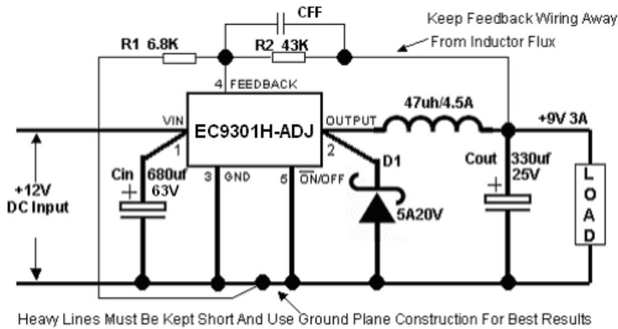
$$V_{out} = V_{ref}(1 + R2/R1) \quad (\text{Where } V_{ref}=1.23V; C_f=1.5nf)$$
