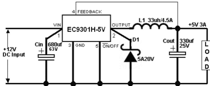
Figure 11. Typical Application of EC9301H For 5V
