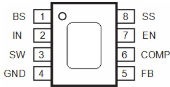
Figure 2 Pin Configuration of EC3283A(Top View)
