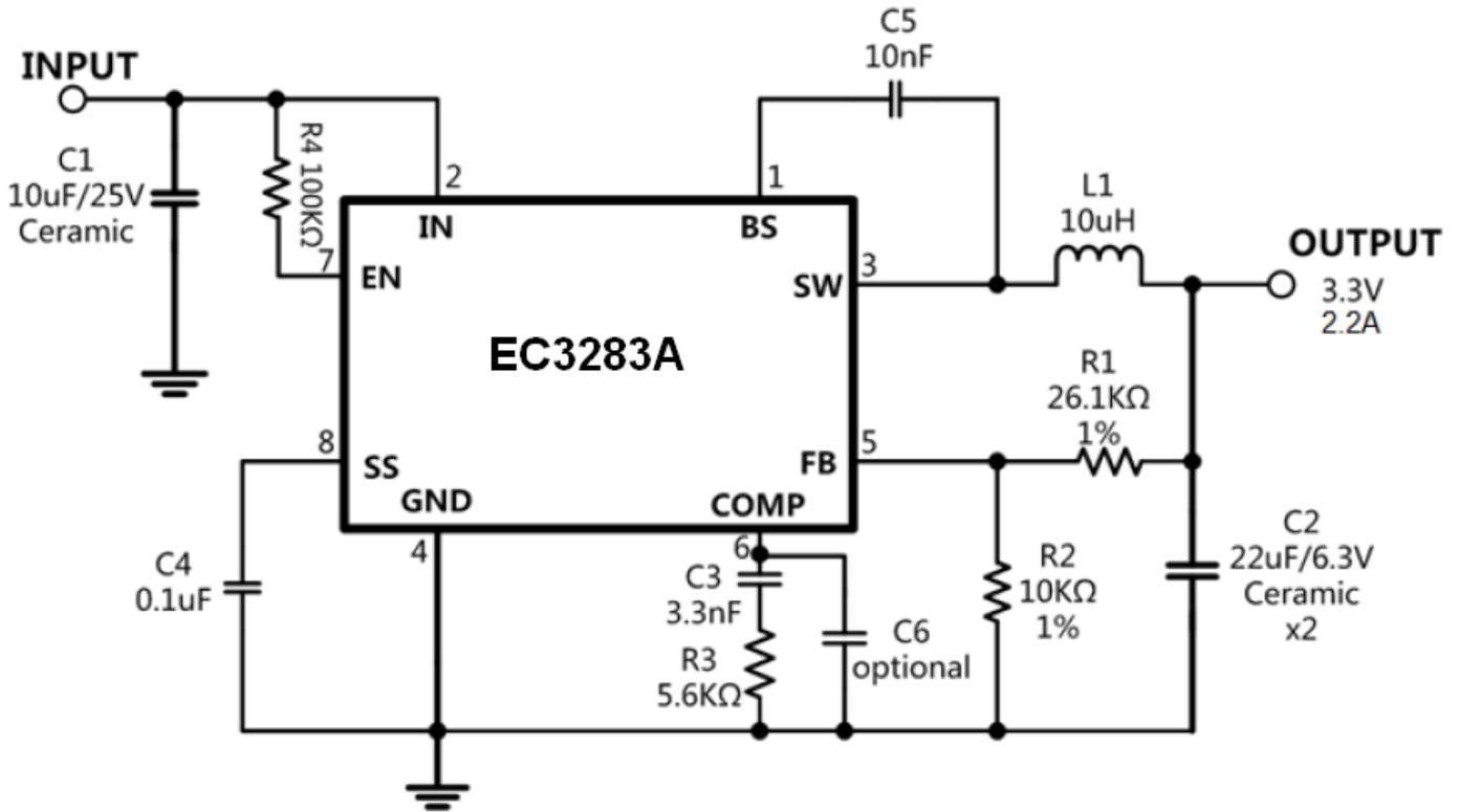
Fig13. EC3283A with 3.3V Output, 22µF/6.3V Ceramic Output Capacitor
