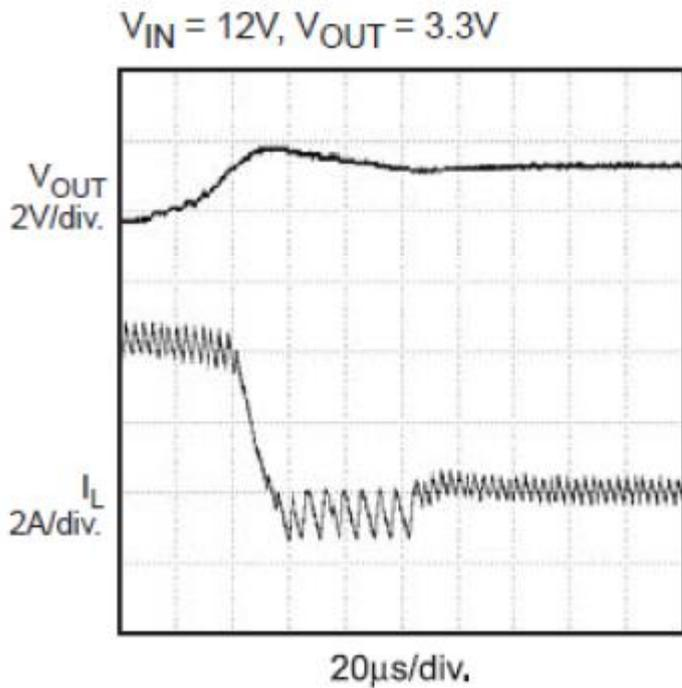
Figure 12. Short Circuit Recovery
