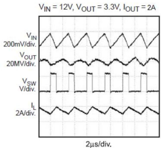
Figure 5. Steady State Test
