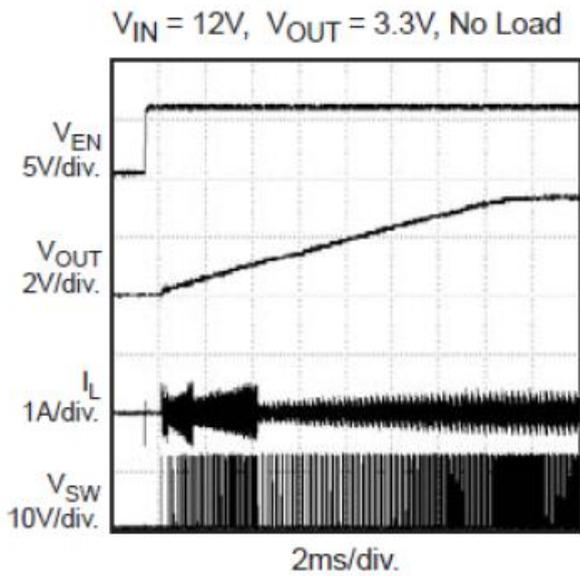
Figure 6. Start up through Enable
