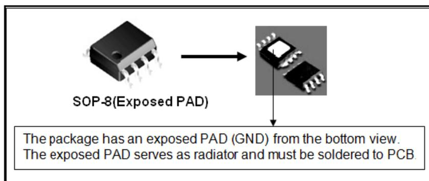
Figure 1. Package Types of EC3283A
