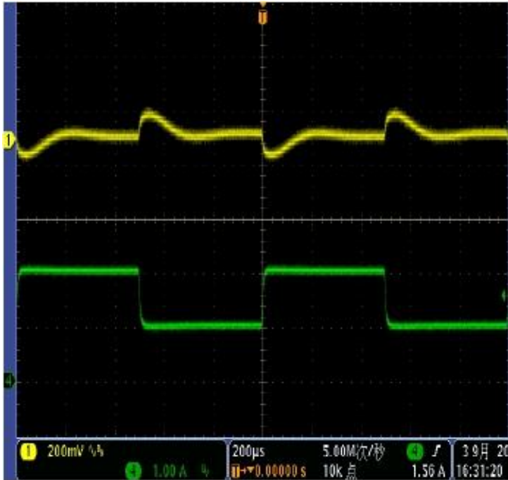
Figure 7. Load Transient Test
